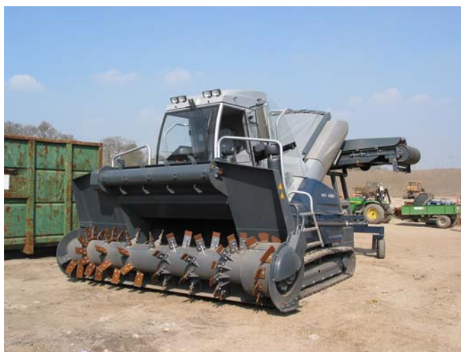
Plate2: Windrow turner (Sandberger UNI 4001) used in enclosed composting hall
